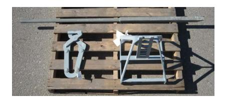
To remove a pin without the use of a hydraulic power pack, there are three tools required in addition to the E-clip tool. They are the pin pulling aid ladder (B990327), the pin puller (B940706), and barrier pulling bar (A990418) which is a specialized pry bar.
